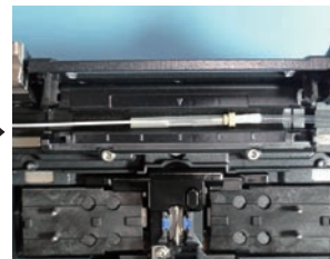
3. protection sleeve shrinking
