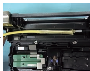
3. protection sleeve shrinking
