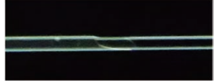
Recoated fiber over coated with 280 mold
